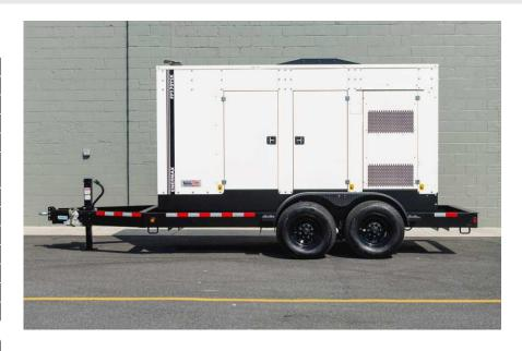
TecnoGen's 170kVA generator uses the FPT engine coupled to an industry standard Leroy Somer alternator producing 132kW of prime power. Standard features include camlocks, block heater and battery charger. The Deep Sea controller makes retrieving vital stats like fuel levels, run time and start logs easy and the sealed doors and 2" thick insulation throughout gives this gen a 70 dBA rating.
