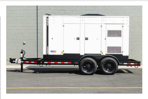
TecnoGen's 225kVA generator uses the FPT engine coupled to an industry standard Leroy Somer alternator producing 181kW of prime power. Standard features include camlocks, block heater and battery charger. The Deep Sea controller makes retrieving vital stats like fuel levels, run time and start logs easy and the sealed doors and 2" thick insulation throughout gives this gen a 70 dBA rating.
