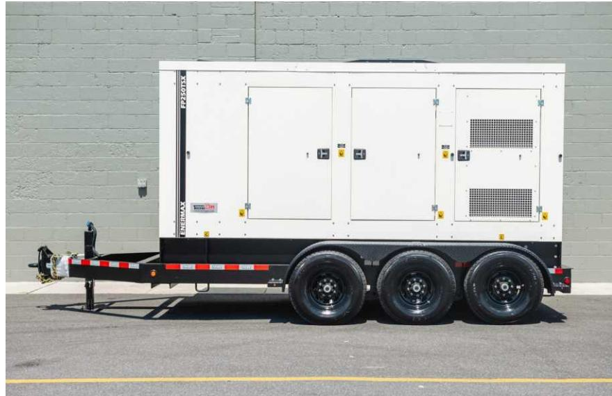
TecnoGen's 250kVA generator uses the FPT engine coupled to an industry standard Leroy Somer alternator producing 201kW of prime power. Standard features include camlocks, block heater and battery charger. The Deep Sea controller makes retrieving vital stats like fuel levels, run time and start logs easy and the sealed doors and 2" thick insulation throughout gives this gen a 70 dBA rating.
