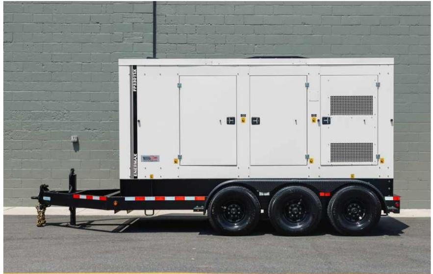
TecnoGen's 330kVA generator uses the FPT engine coupled to an industry standard Leroy Somer alternator producing 263kW of prime power. Standard features include camlocks, block heater and battery charger. The Deep Sea controller makes retrieving vital stats like fuel levels, run time and start logs easy and the sealed doors and 2" thick insulation throughout gives this gen a 70 dBA rating.
