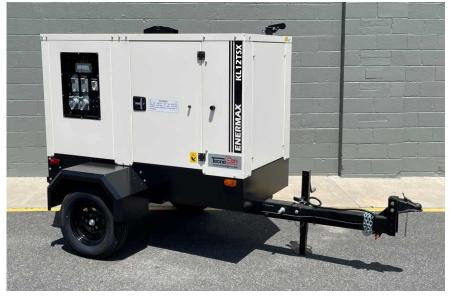
TecnoGen's 12kVA generator uses the Kohler engine coupled to an industry standard Leroy Somer alternator producing 10kW of prime power. Standard features include camlocks and block heater. The Deep Sea controller makes retrieving vital stats like fuel levels, run time and start logs easy and the sealed doors and 2" thick insulation throughout gives this gen a 68 dBA rating.
