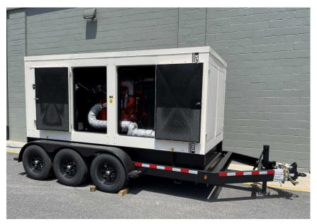
TecnoGen's 300kVA generator uses the Scania engine coupled to an industry standard Leroy Somer alternator producing 240kW of prime power. Standard features include camlocks, block heater and battery charger. The Deep Sea controller makes retrieving vital stats like fuel levels, run time and start logs easy and the sealed doors and 2" thick insulation throughout gives this gen a 70 dBA rating.
