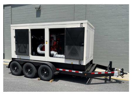
TecnoGen's 420kVA generator uses the Scania engine coupled to an industry standard Leroy Somer alternator producing 334kW of prime power. Standard features include camlocks, block heater and battery charger. The Deep Sea controller makes retrieving vital stats like fuel levels, run time and start logs easy and the sealed doors and 2" thick insulation throughout gives this gen a 70 dBA rating.
