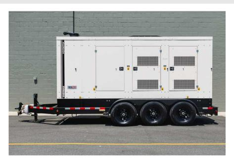
TecnoGen's 700kVA generator uses the Volvo engine coupled to an industry standard Leroy Somer alternator producing 560kW of prime power. Standard features include camlocks, block heater and battery charger. The Deep Sea controller makes retrieving vital stats like fuel levels, run time and start logs easy and the sealed doors and 2" thick insulation throughout gives this gen a 71 dBA rating.
