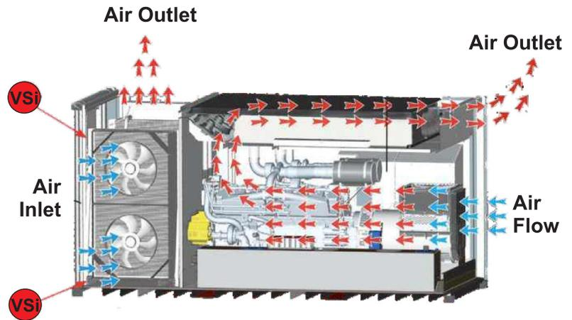
The FQ series generators by TecnoGen incorporate their Patented VSi technology. VSi (Variable Speed inverter) technology uses variable speed electric fans to manage the cooling for the generator instead of standard engine driven fans, which steal power from the engine and create excessive noise.
