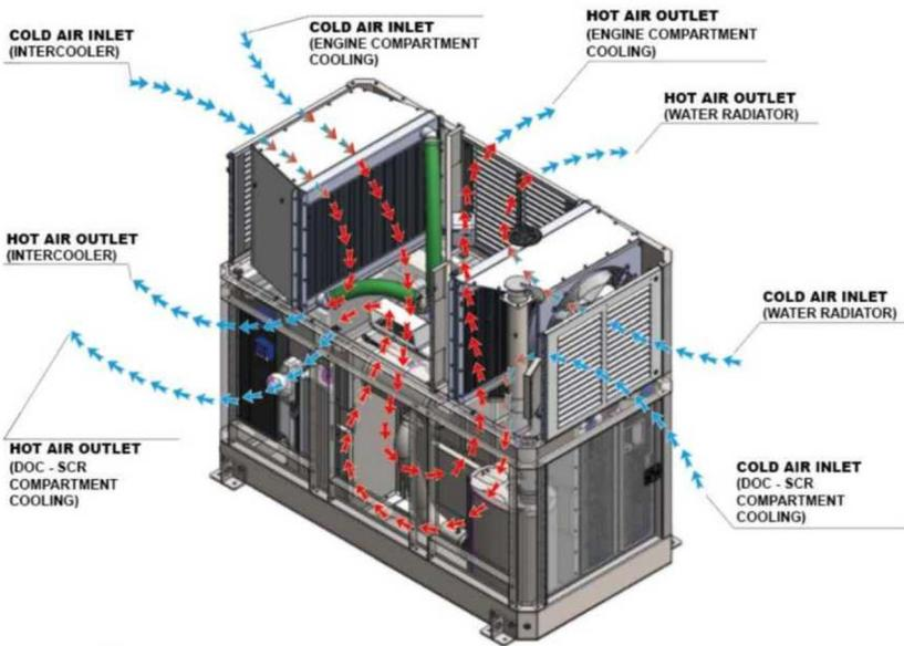
The Movie Master series generators by TecnoGen incorporate their patented VSi technology. VSi (Variable Speed inverter) technology uses variable speed electric fans to manage the cooling for the generator instead of standard engine driven fans, which steal power from the engine and create excessive noise. Standard fans require more horsepower and consume 3 GPH more fuel than TecnoGen VSi cooled units.
